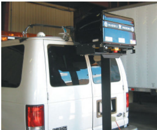
Figure 2. PPS device mounted on Iowa DOT video log van
