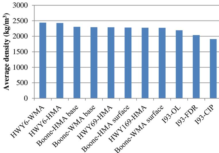
**Figure 4.4. Comparison of average CoreLok densities from 11 sections**
