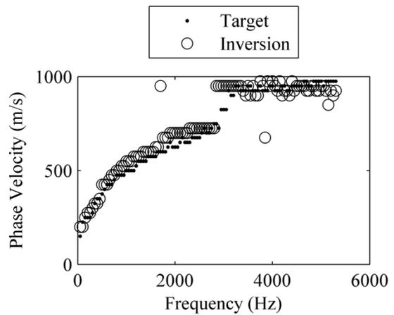
**Figure A.21. Picked experimental dispersion curves (targets), and theoretical dispersion curves from inversion for cold tests on IA 93 CIP and OL sections after applying dry ice**
