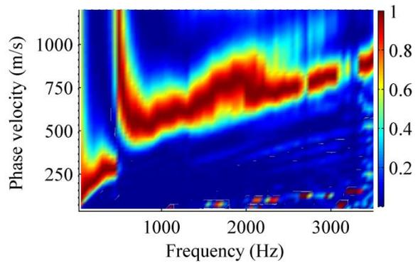
**Figure A.7. Results of surface wave tests on ambient-temperature Boone HMA surface courses one day after paving. Left column: normalized time-domain signals, right column: frequency-domain dispersion images**
