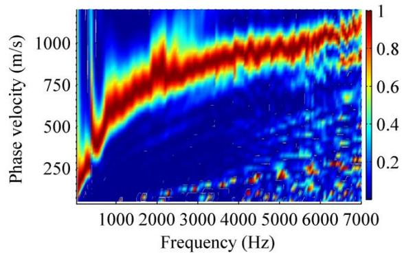
**Figure A.8. Results of surface wave tests on ambient-temperature Boone WMA surface courses one day after paving. Left column: normalized time-domain signals, right column: frequency-domain dispersion images**
