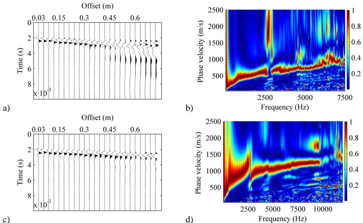
**Figure 3.7. MSOR surface-wave test results for location US 169-4: (a) normalized time-domain data for cold test after dry ice, (b) experimental dispersion trend for cold test after dry ice, (c) normalized time-domain data for ambient-temperature test four days after paving, (d) experimental dispersion trend for ambient-temperature test four days after paving**
