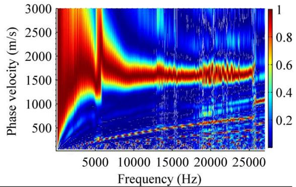
**Figure A.24. Results of surface wave tests on ambient-temperature US 6 HMA surface course several days after paving. Left column: normalized time-domain signals, right column: frequency-domain dispersion images**
