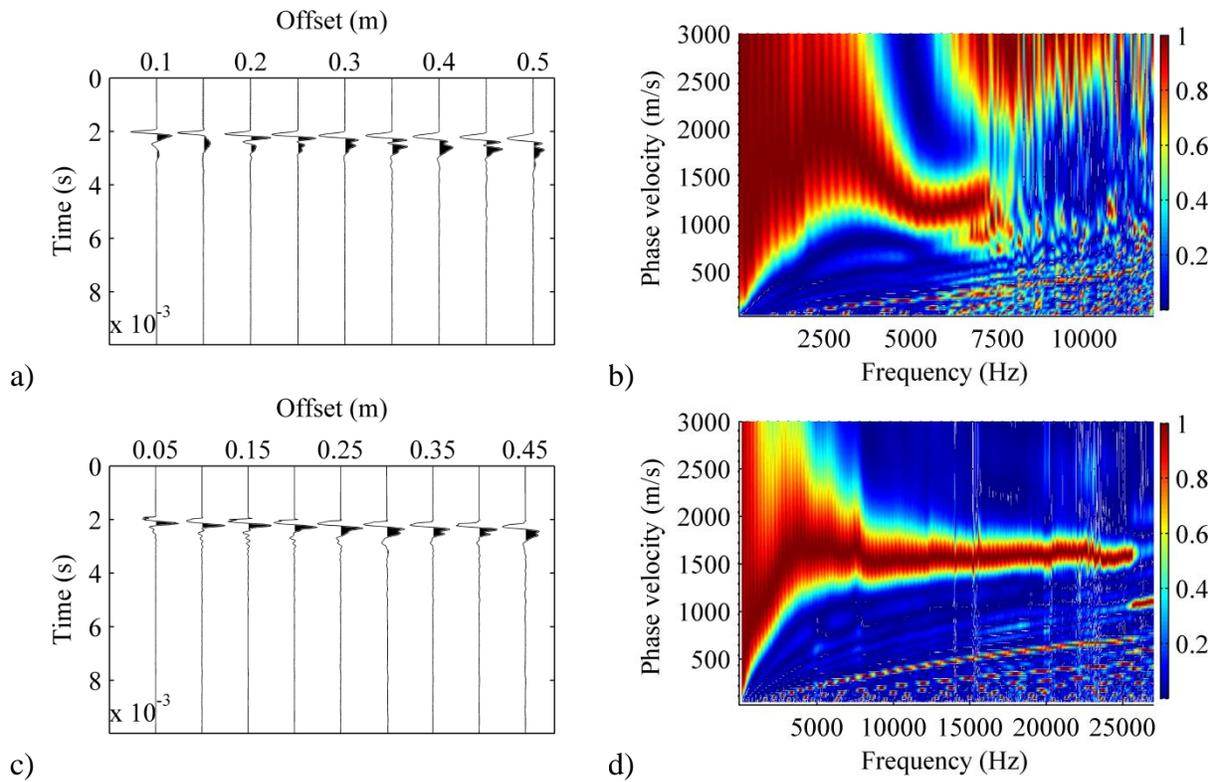
**Figure 3.11. MASW surface-wave tests on US 6 W30-2: (a) normalized time-domain data for hot test, (b) experimental dispersion trend for hot test, (c) normalized time-domain data for ambient-temperature test, (d) experimental dispersion trend for ambient-temperature test**
