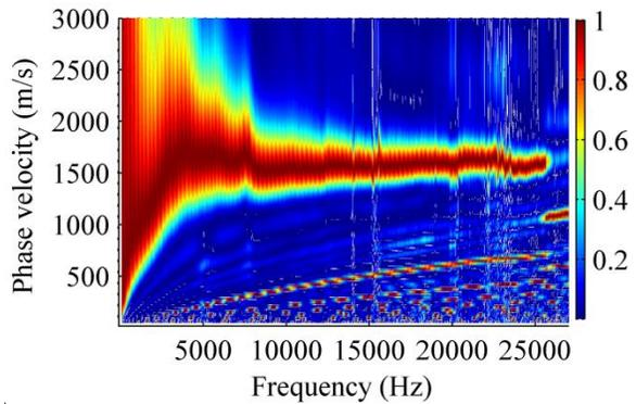
**Figure A.25. Results of surface wave tests on ambient-temperature US 6 WMA surface course several days after paving. Left column: normalized time-domain signals, right column: frequency-domain dispersion images**
