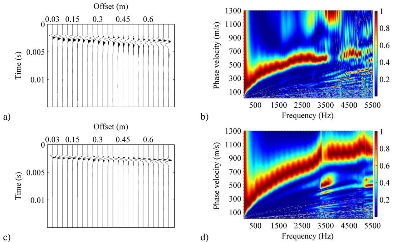
**Figure 3.9. MSOR surface-wave tests on IA 93-OL1: (a) normalized time-domain data for hot test, (b) experimental dispersion trend for hot test, (c) normalized time-domain data for cold test, (d) experimental dispersion trend for cold test**
