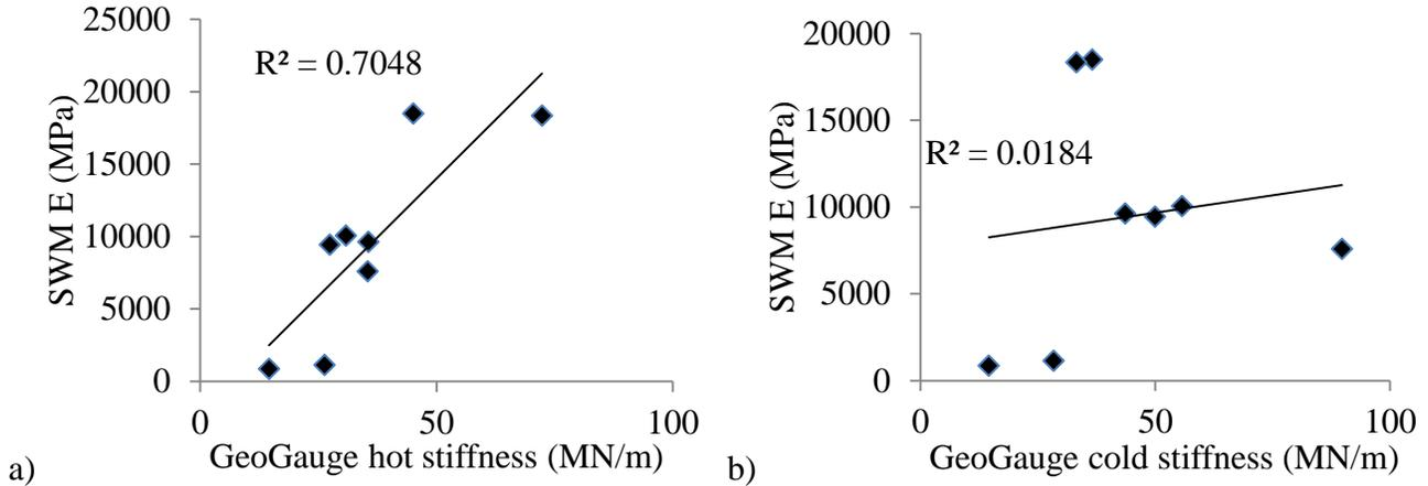
**Figure 5.4 Correlation between GeoGauge stiffness and SWM cold/ambient modulus: (a) hot GeoGauge tests and (b) cold/ambient GeoGauge tests**
