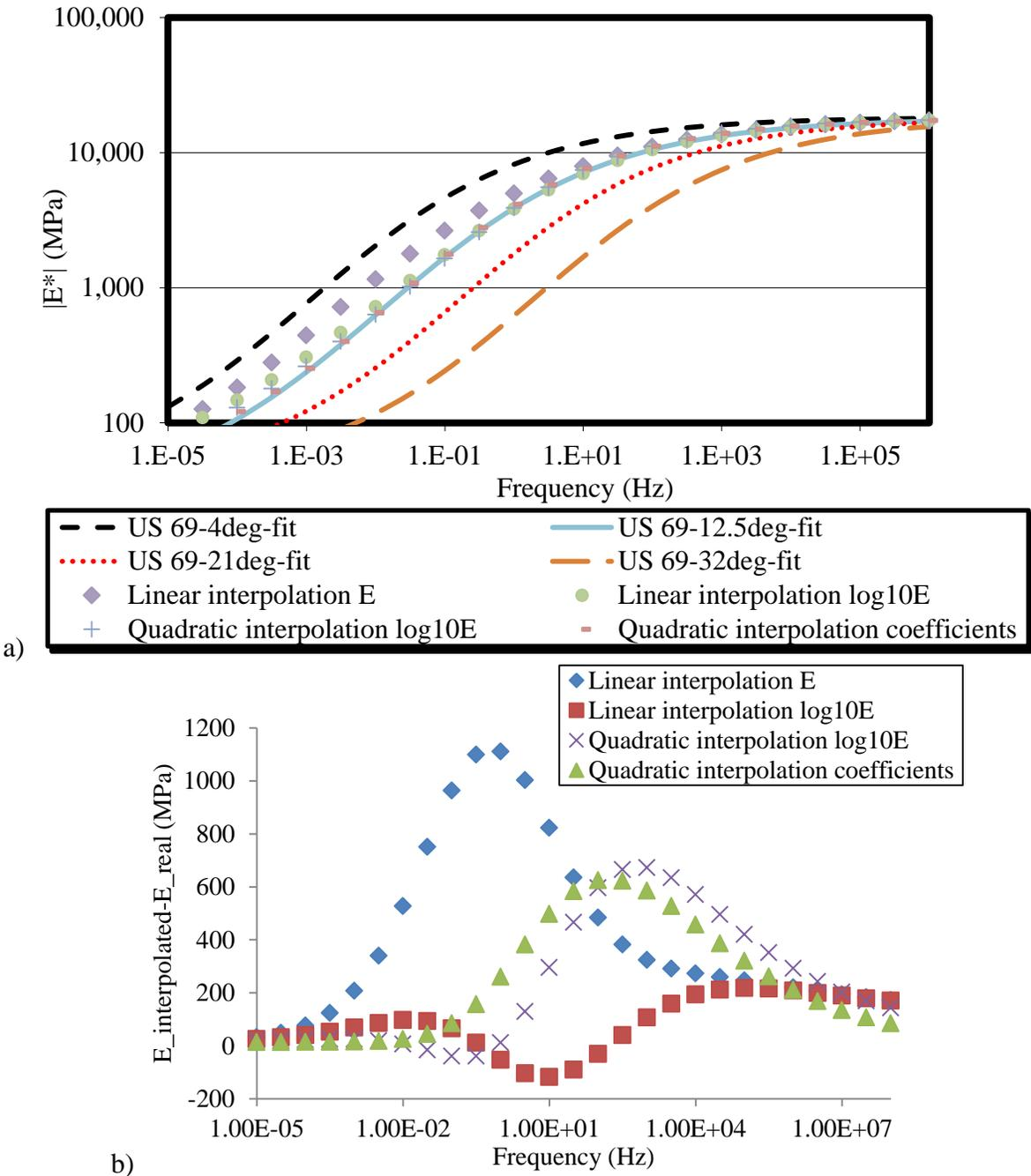
**Figure 4.11. Interpolation of master curves at a reference temperature of 12.5°C: (a) four measured and four interpolated master curves, and (b) discrepancy between interpolated and measured master curves versus frequency**
