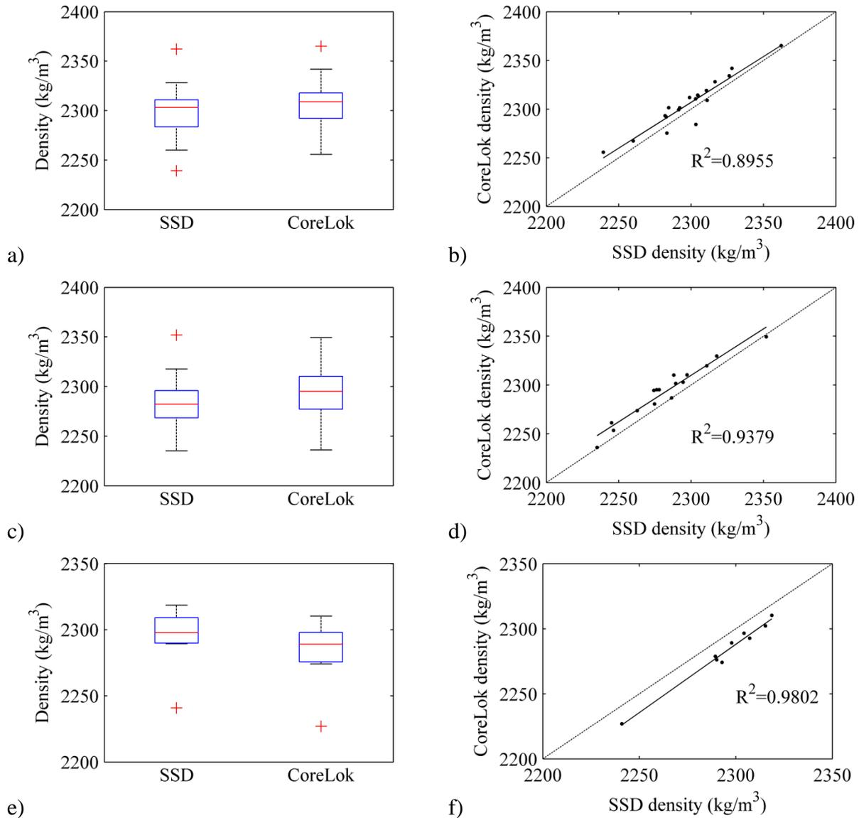
**Figure 4.2. Comparison of SSD and CoreLok densities for 19 Boone HMA base course cores: (a) boxplot and (b) correlation; 16 Boone WMA base course cores: (c) boxplot and (d) correlation; 9 US 69 surface course cores: (e) boxplot and (f) correlation**
