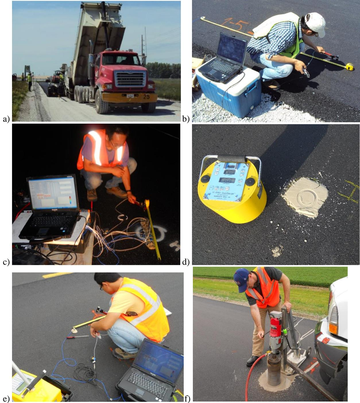
**Figure 3.2. (a) Pavement construction at Central Iowa Expo site, (b) MSOR surface-wave testing at Central Iowa Expo site, (c) MASW surface wave testing on US 6, (d) GeoGauge testing on IA 93, (e) MSOR surface-wave testing on US 69, (f) coring on US 69**
