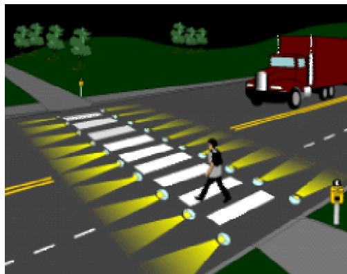
Figure 1. In-pavement flashing warning lights (walkinginfo.org)
