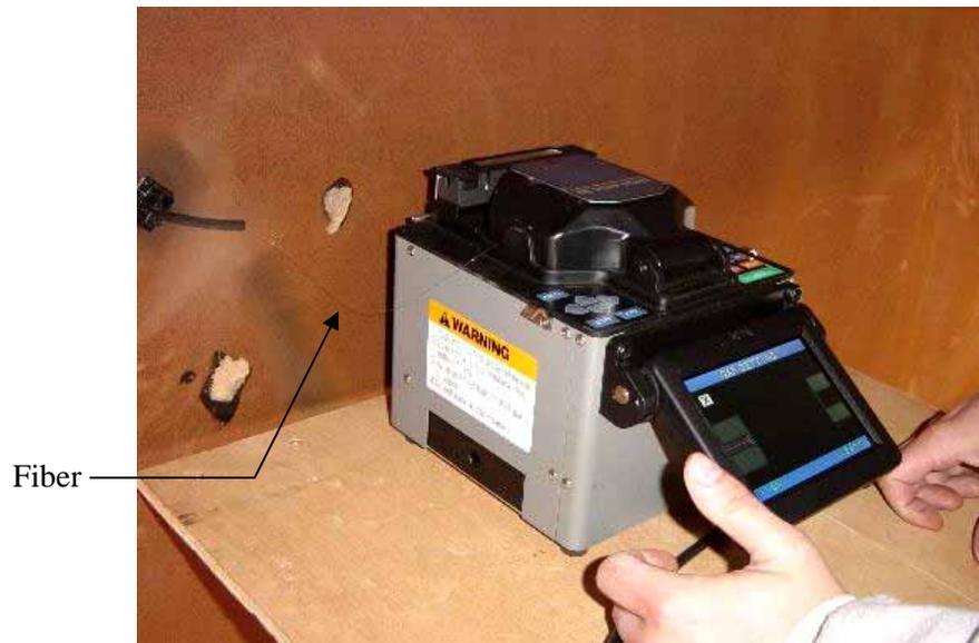
**Figure 4.11. Fusion splicing of two fibers**
