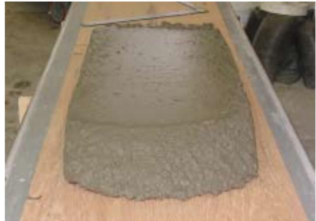
*Test section of SCC extruded from mini-paver*
