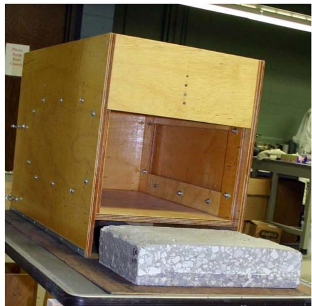
*Mini-paver with section of SCC pavement slab*
