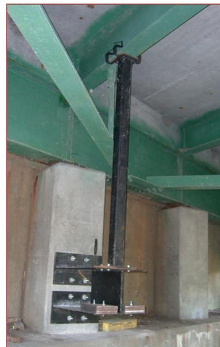
*Typical installed sacrificial specimen*
