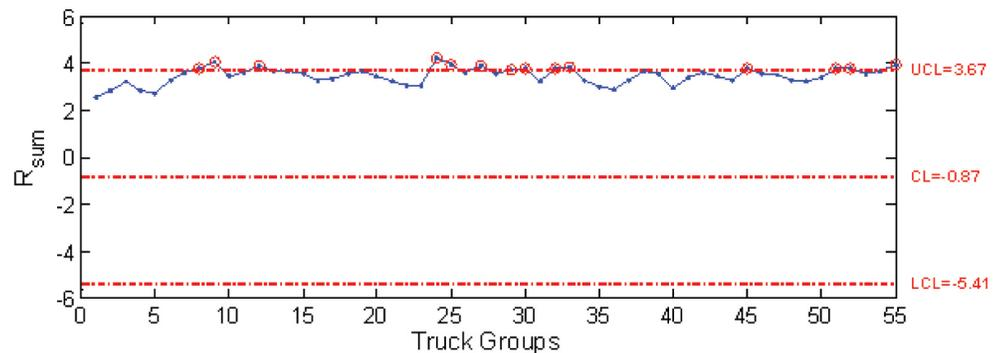
Sample control chart indicating damage detection (red-circled data points above the upper control limit (UCL))
