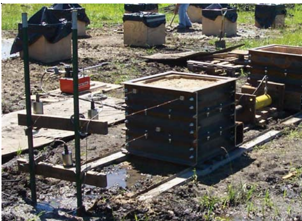
Large-scale direct shear test setup
