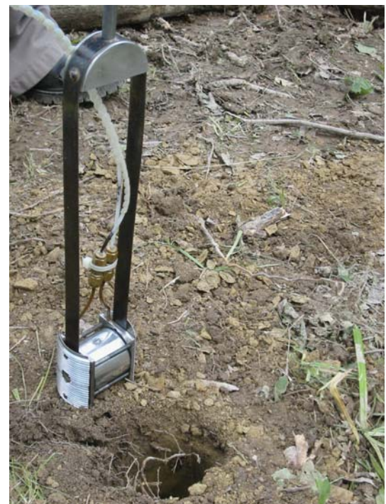
Iowa BST device: shear head
