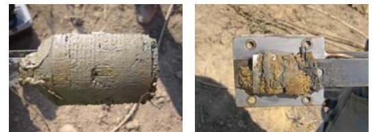
Iowa BST shear plates after shearing: normal shear plates (left) and high stress shear plates (right)
