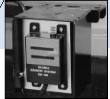
reverse obstacle sensors: Global Sensor Systems Ontario, Canada
