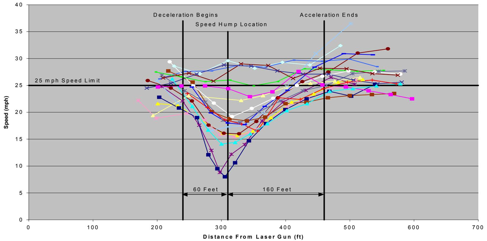
Figure 35. Roosevelt Drive Southbound Speed Hump Spacing Analysis
