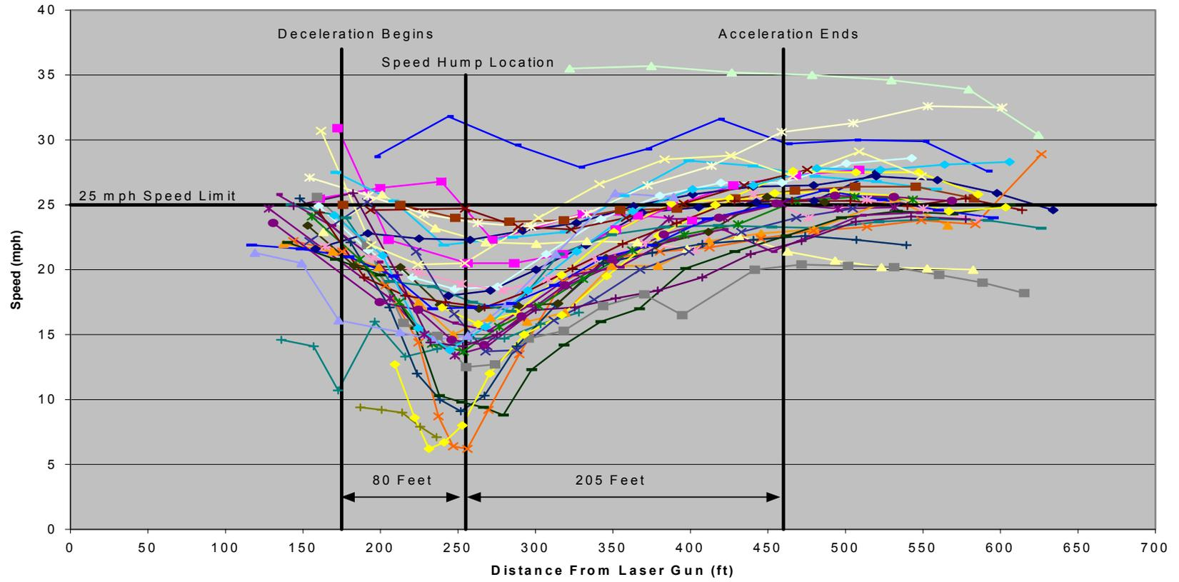
Figure 36. Redwood Drive Speed Hump Spacing Analysis
