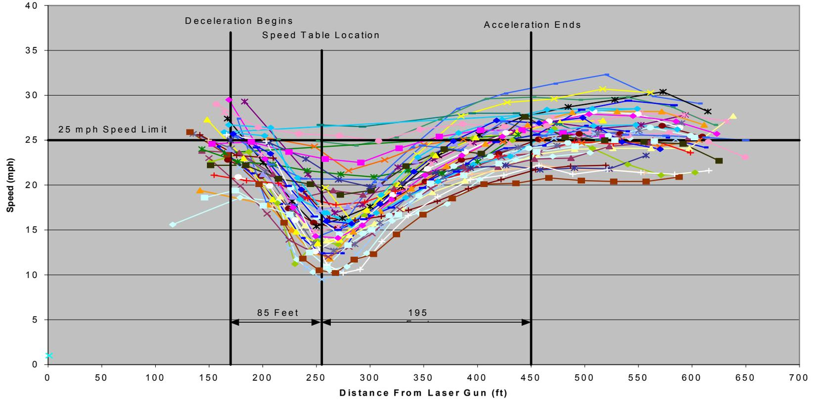
Figure 37. Redwood Drive Speed Table Spacing Analysis
