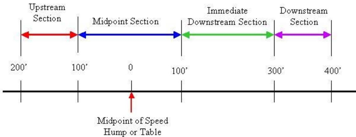
**Figure 30. Schematic of Section Locations**
