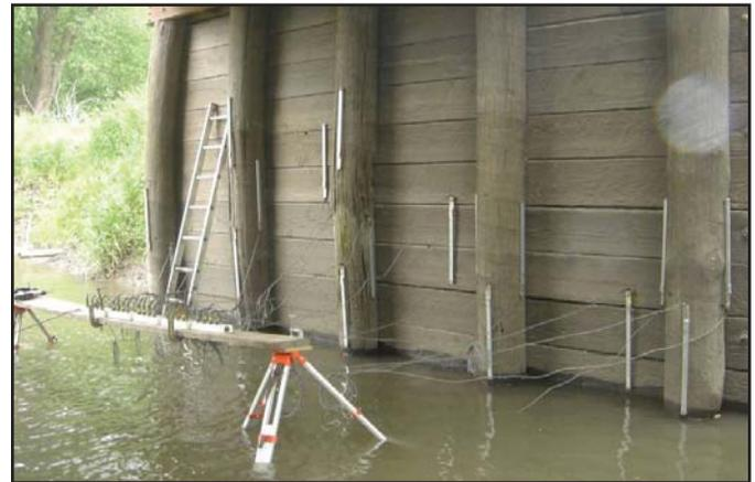
*Bridge abutment instrumented with strain gauges*
