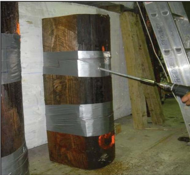
*Timber pile repair using mechanical splicing*
