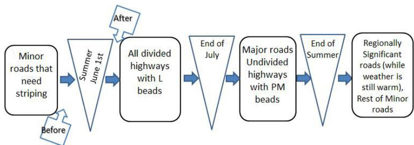
*MoDOT striping plan starting in 2015 (with the introduction of a new type of beads for divided highways that require higher drying temperatures)*
