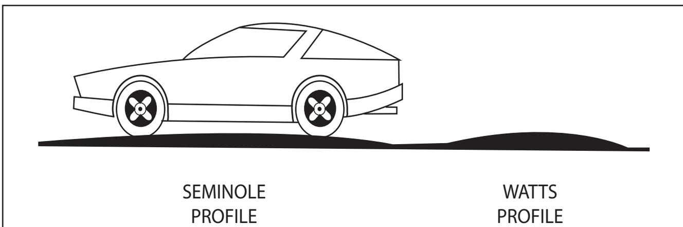
*Diagram illustrating the difference between a Seminole profile speed table and a traditional Watts profile speed hump*
