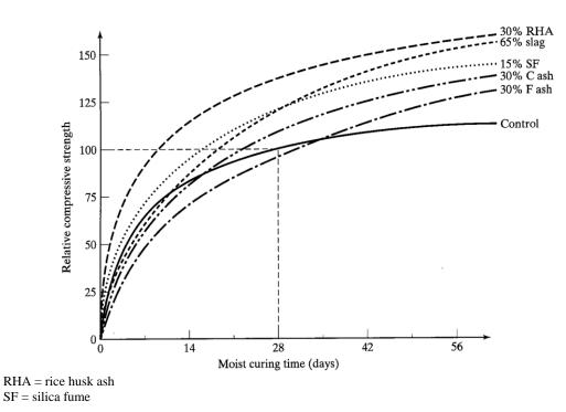
Figure 3. Relationship between relative compressive strength and supplementary cementitious materials [8]
