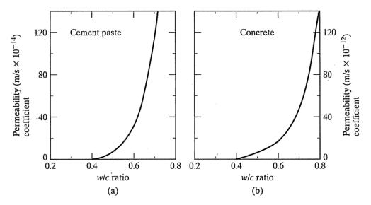
Figure 5. Influence of w/c on the permeability of (a) cement paste and (b) concrete [9]
