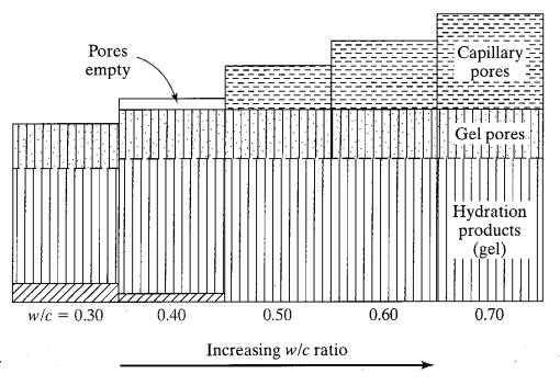
Figure 2. Relationship between porosity and w/c [8]
