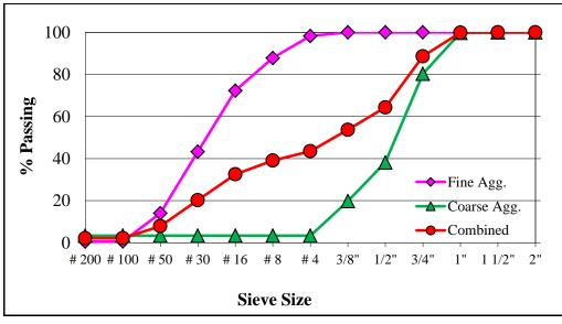
c) ASTM C33 gradation graph
