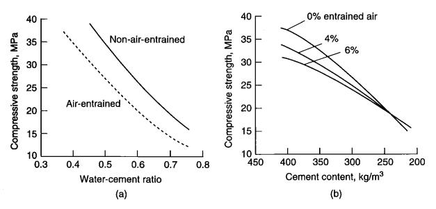
Figure 4. Influence of entrained air on compressive strength [4]
