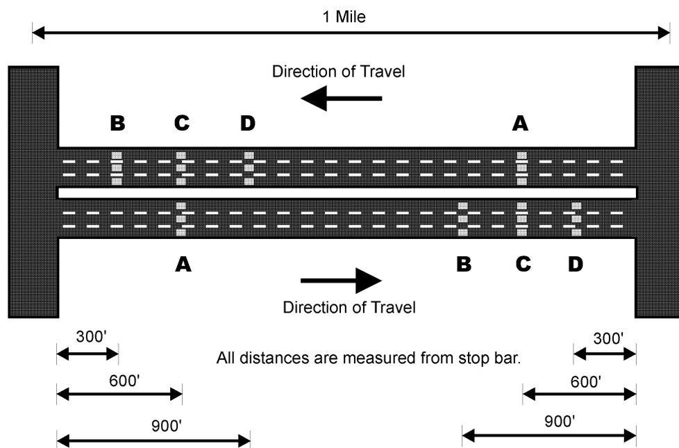
FIGURE 2 Surveillance detector locations
