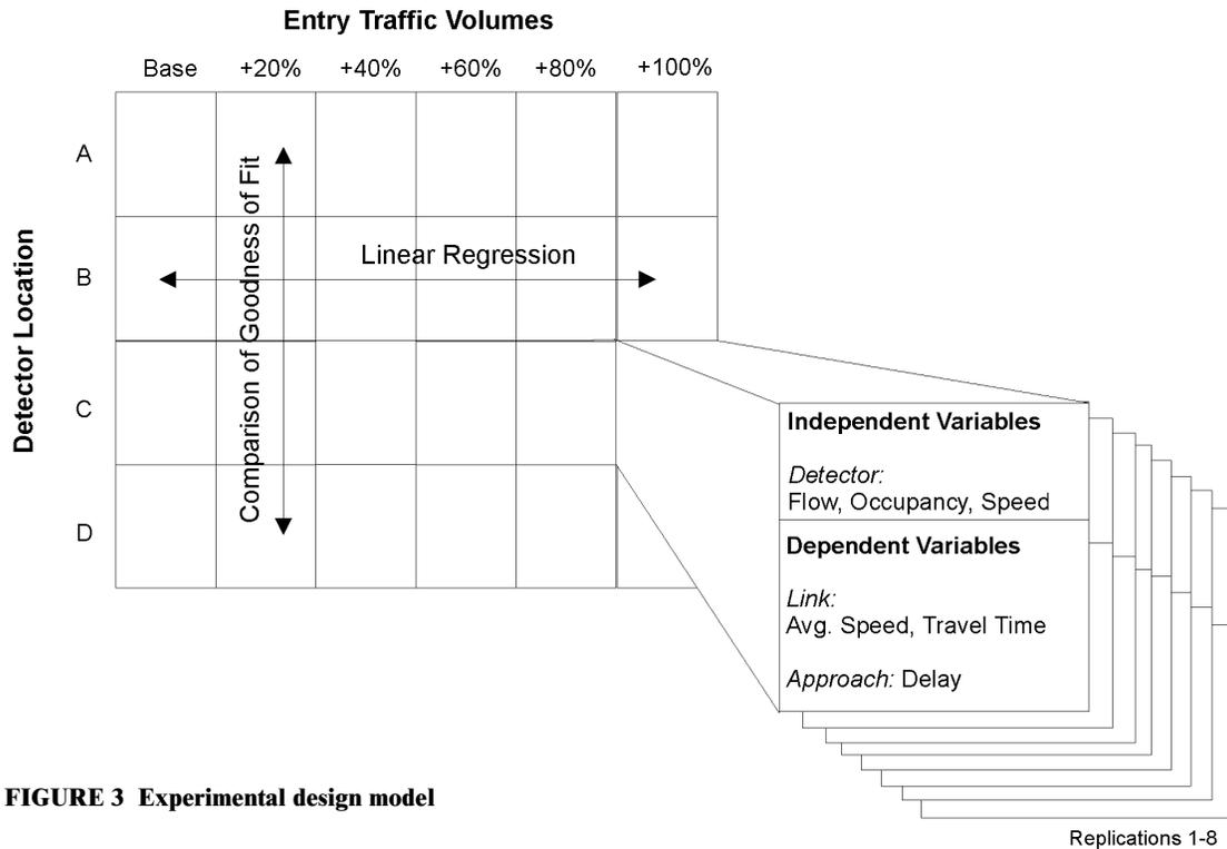
**FIGURE 3** Experimental design model
