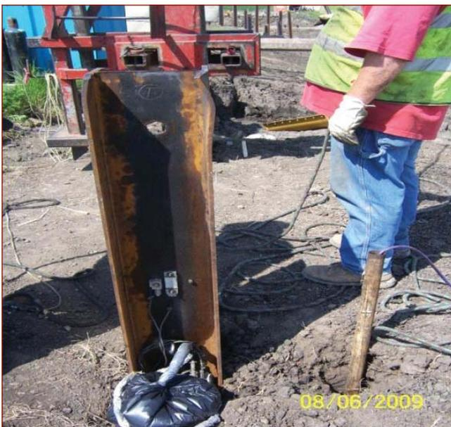
Pore water and lateral earth pressure measurement
