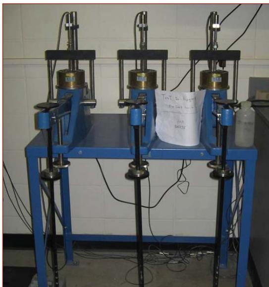
*Laboratory soil tests (consolidation test)*
