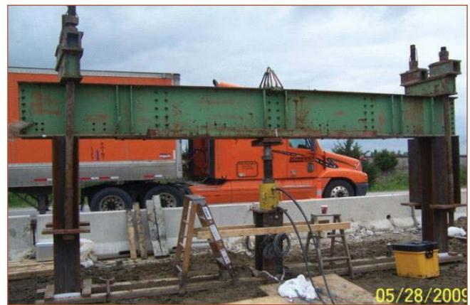
Completed static load test frame
