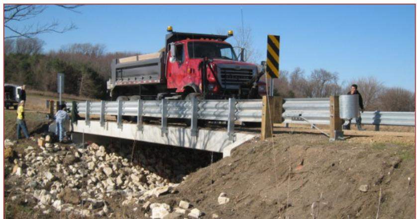
Load testing the completed, single-span, 50 ft (center to center of supports), Buena Vista County IBRD bridge
