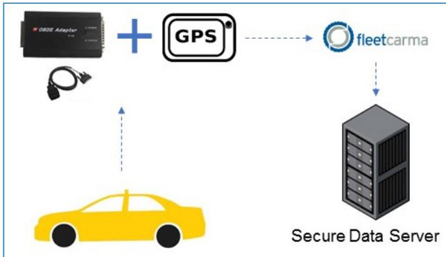
*Vehicle controller area network (CAN) bus data collection*
