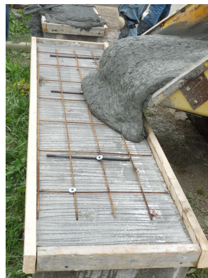
Concrete slab specimen with wire mesh being overlaid with UHPC
