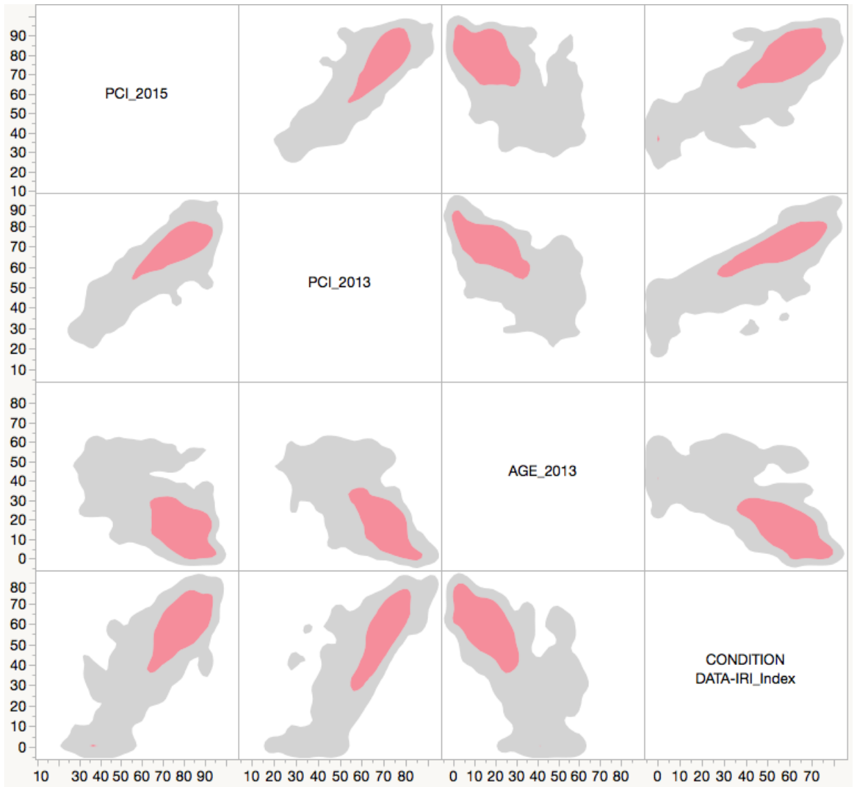
Figure 2. Selected scatter plots showing how four variables interact to predict PCI_2015 for Pavement Type 1
