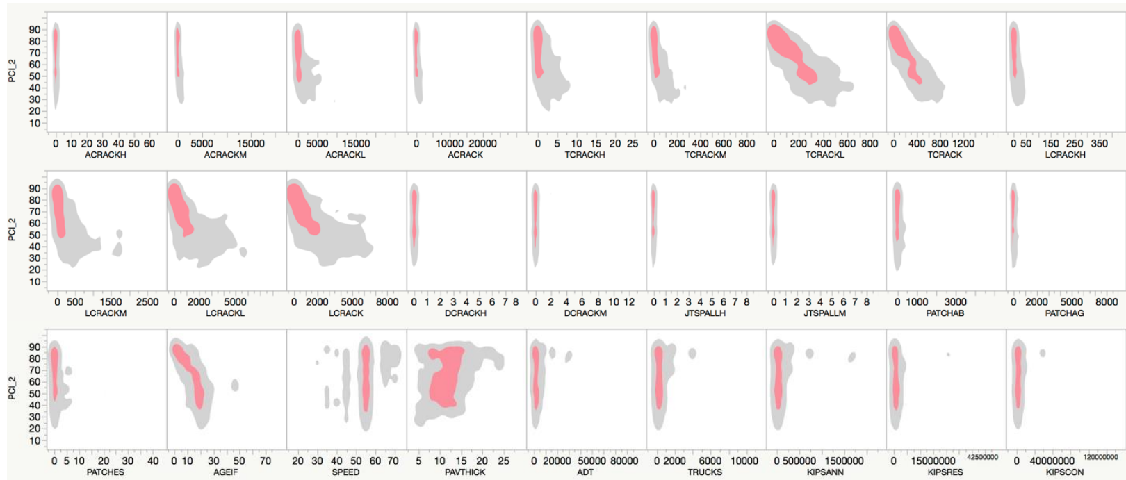
Figure 3. Scatter plots showing how 27 measures and variables interact with PCI for Pavement Type 4
