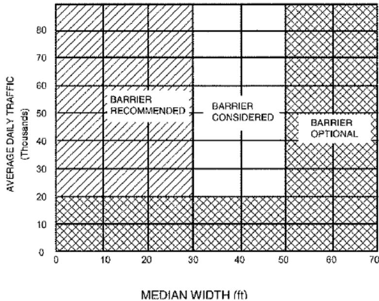
**Figure 2. AASHTO *Roadside Design Guide* barrier guidance**
