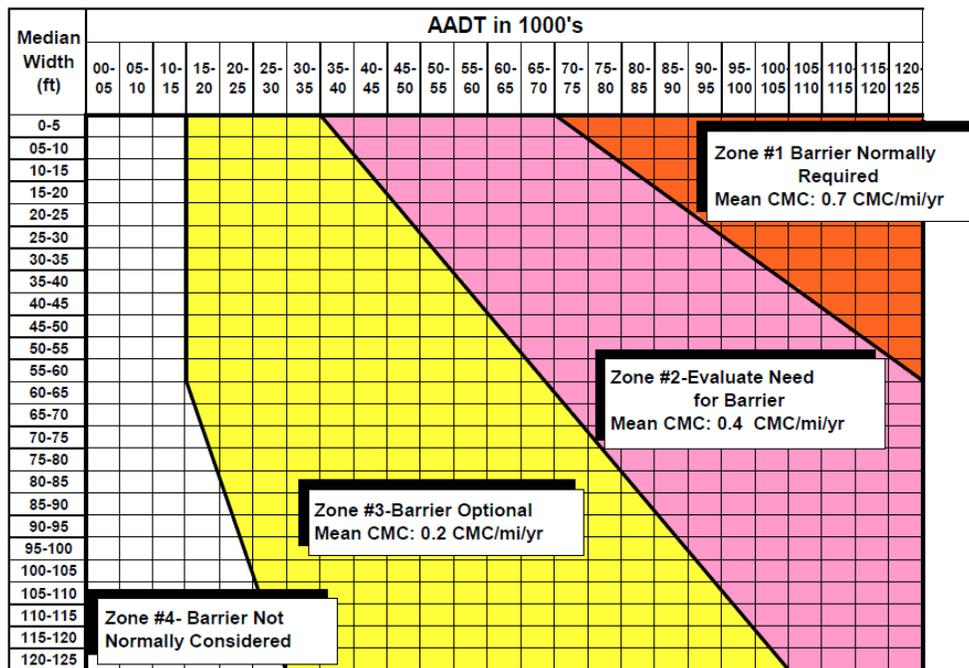
Figure 3. Texas-specific guidelines for installing median barriers
