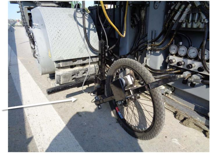
Distance measuring device (DMI) connected and clear from paver track line obstructions
