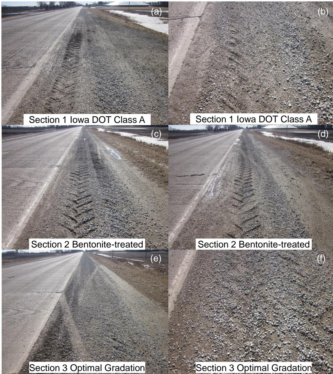
**Figure 4.45. Survey photos of T Ave. shoulder test sections taken during thawing period on February 12, 2017**
