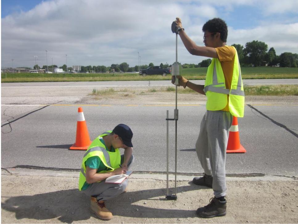
**Figure 4.4. DCP test performed on the Highway 30 off-ramp shoulder section**
