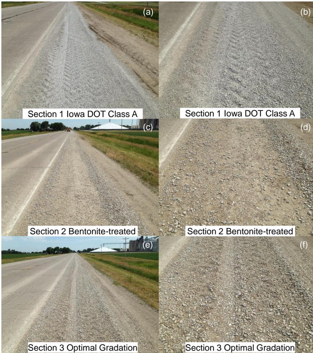
**Figure 4.42. Survey photos of T Ave. shoulder test sections taken on June 24, 2016**
