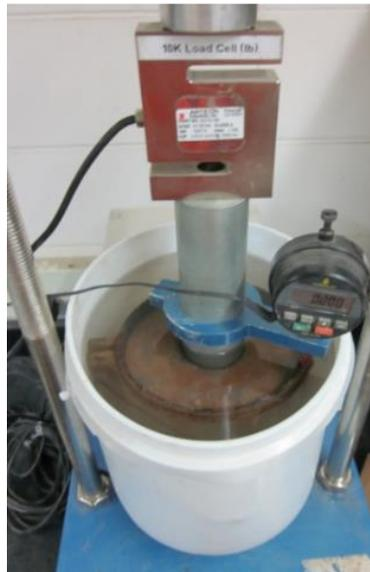
**Figure 3.2. CBR test conducted on soaked specimens**
