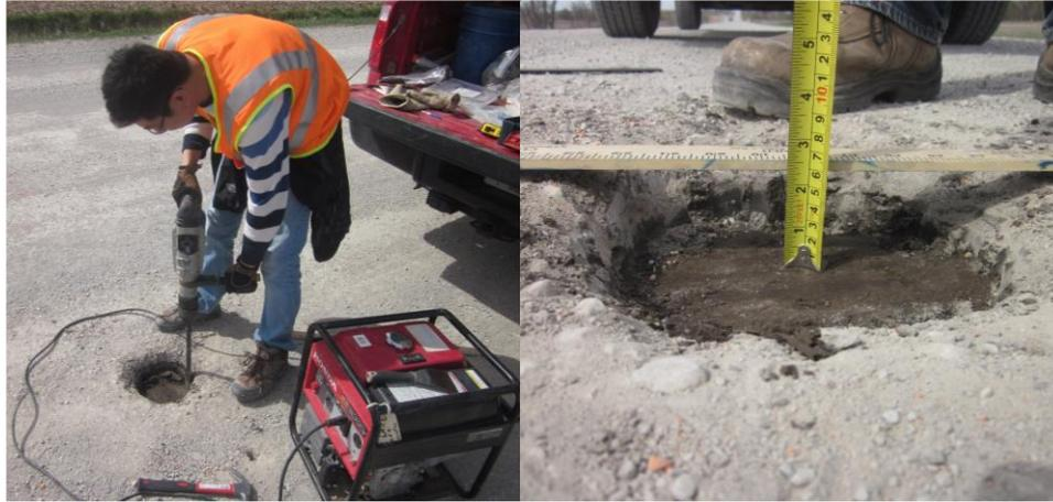
**Figure 4.12. Excavation performed on the test section to measure thickness of surface layer and identify the source of excessive fines**
