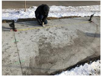
Measurements to monitor deflection/slab surface profile over time
