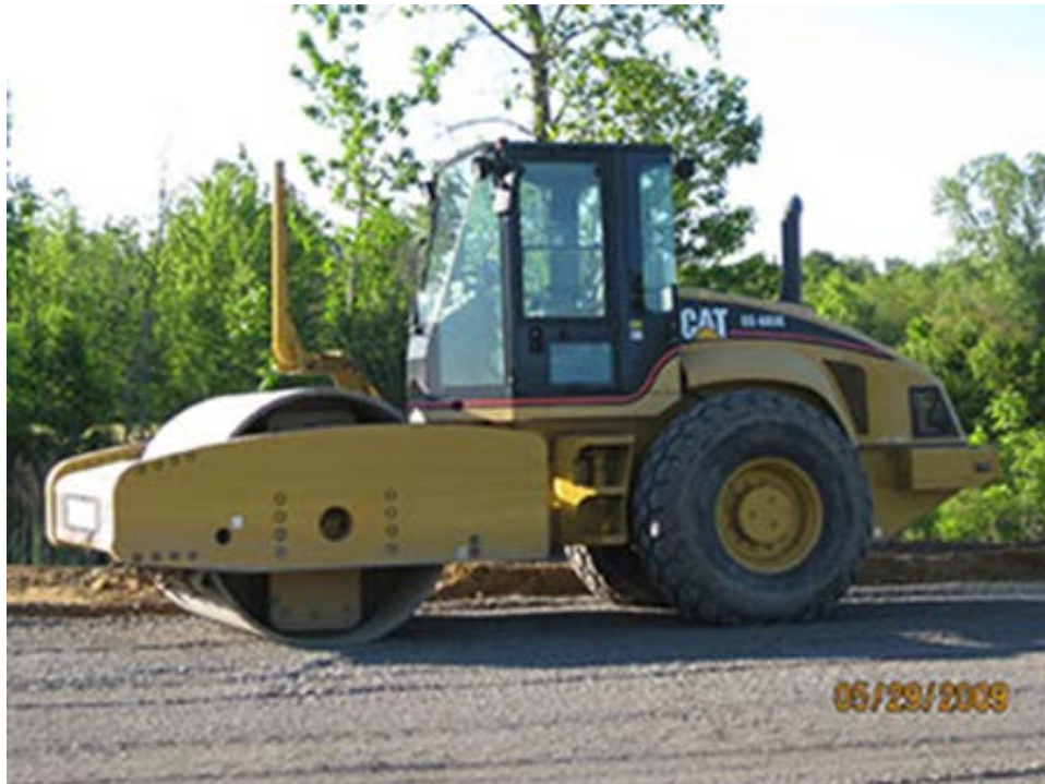
Figure 26. Caterpillar CS683 vibratory smooth drum IC roller
