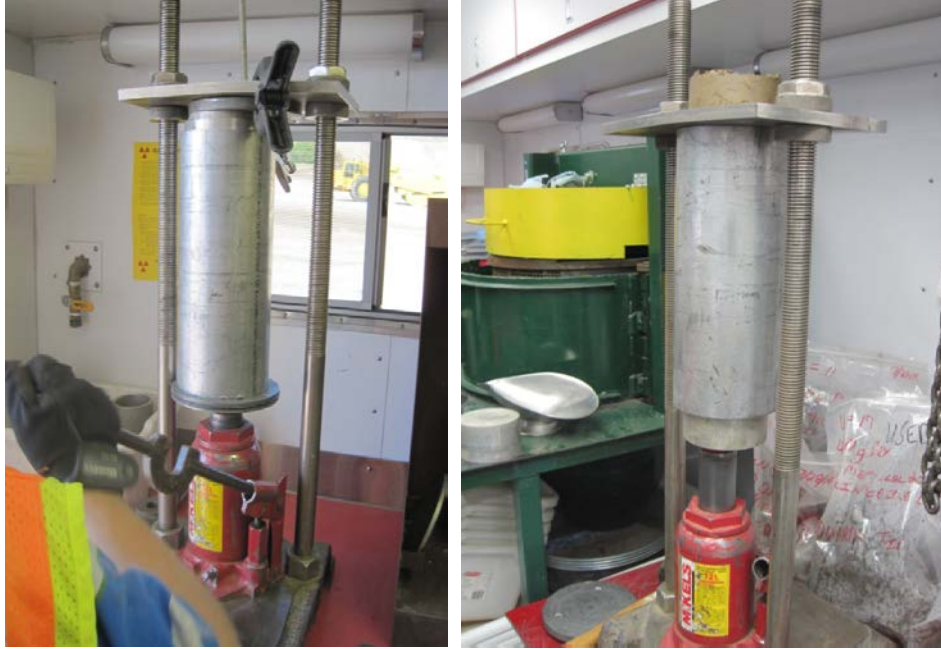
Figure 14. Photos showing static compaction procedure (left) and sample extrusion procedure (right) of a compacted cohesive soil sample
