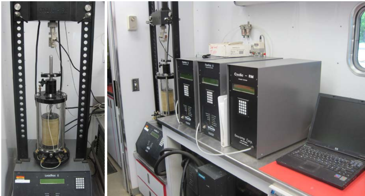
Figure 18. Triaxial chamber, load frame, and computer equipment for resilient modulus tests
