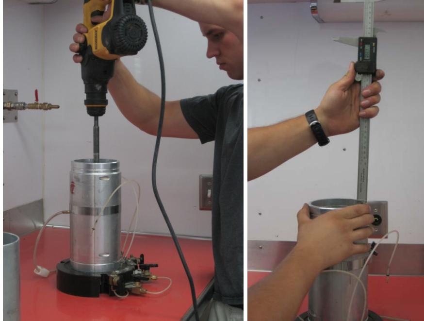
Figure 11. Compaction of granular materials in split mold and verification of thickness of each lift using calipers
