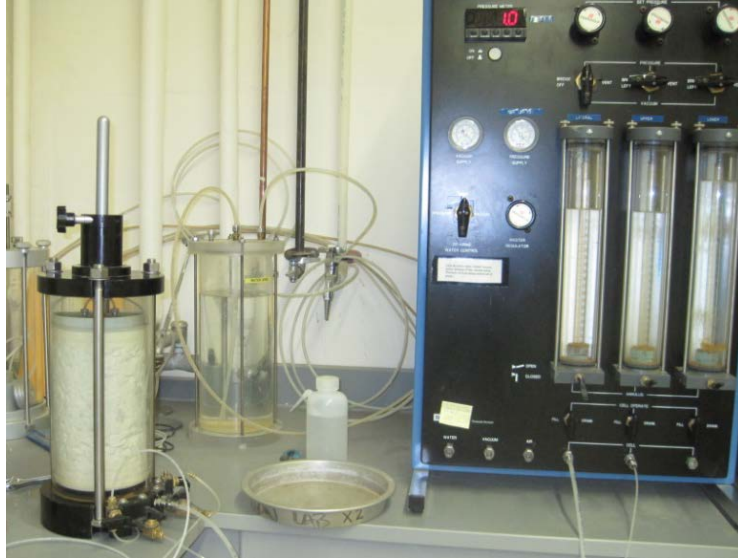
Figure 17. Sample in a triaxial cell and pressure control wall used in back saturation prior to M_r testing
