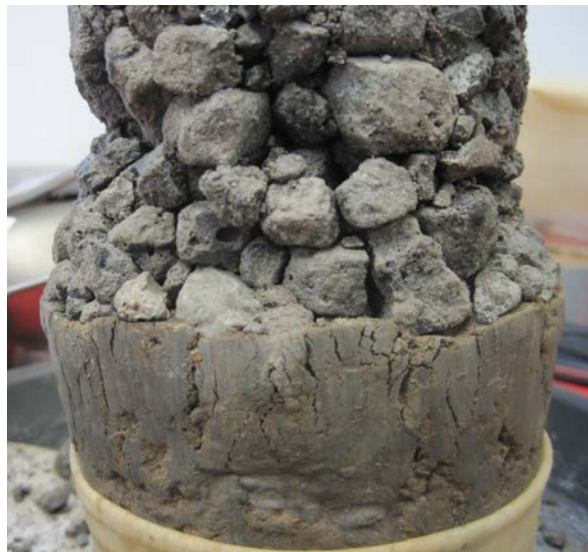
Figure 40. Untrimmed base ( 16.65 \text{ kN/m}^3 at 1.6% moisture) over subgrade ( 17.37 \text{ kN/m}^3 at 15.0% moisture) after M_r testing
