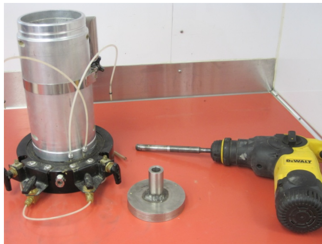
Figure 10. Split mold, steel platen (4 in. diameter), and vibratory hammer for compaction of granular materials
