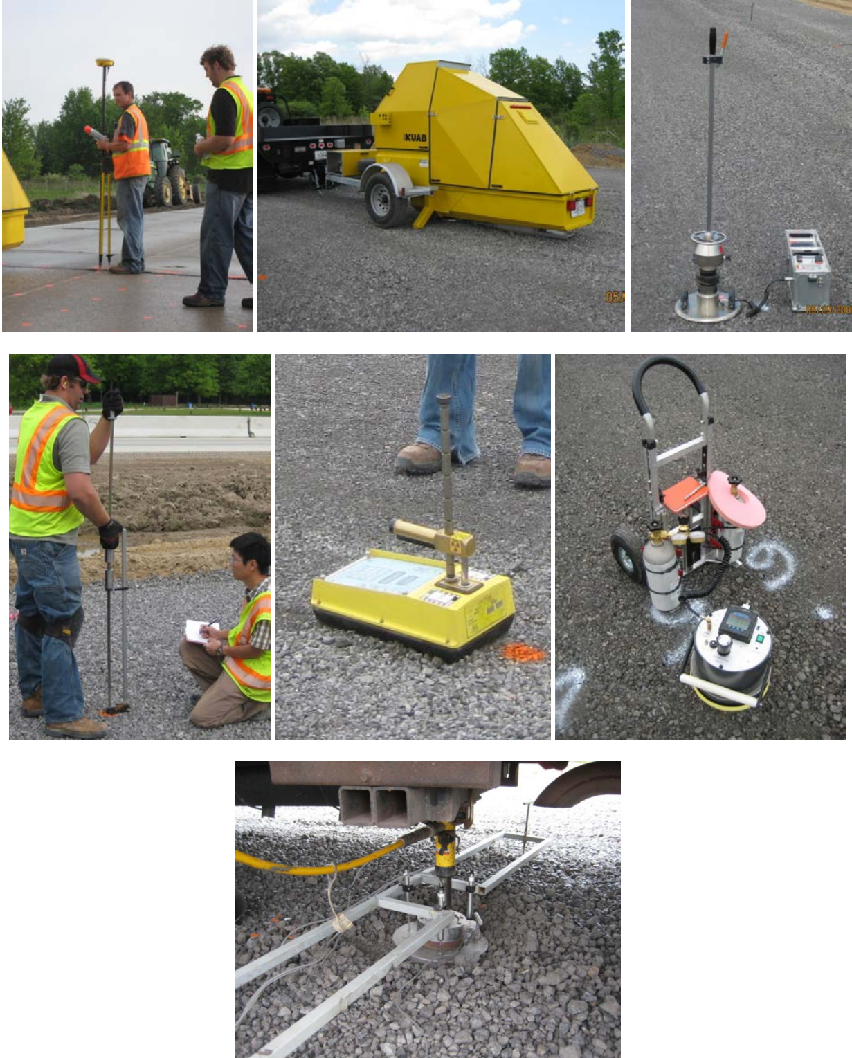
Figure 22. Trimble SPS-881 hand-held receiver, Kuab falling weight deflectometer, and Zorn light weight deflectometer (top row left to right); dynamic cone penetrometer, nuclear gauge, and gas permeameter device (middle row left to right); static plate load test (bottom row)
