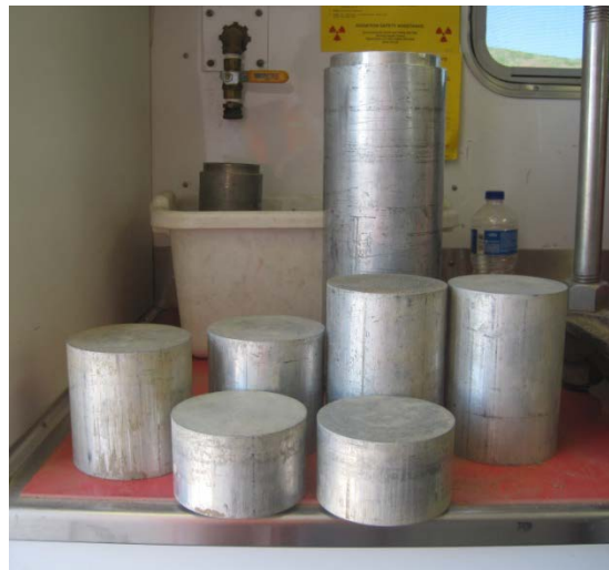
Figure 13. Aluminum spacers (4 in. diameter) used during static compaction
