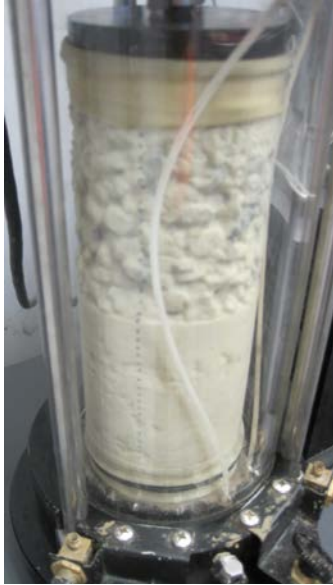
Figure 39. Untrimmed base ( 16.65 \text{ kN/m}^3 at 1.6% moisture) over subgrade ( 17.37 \text{ kN/m}^3 at 15.0% moisture) during M_r testing
