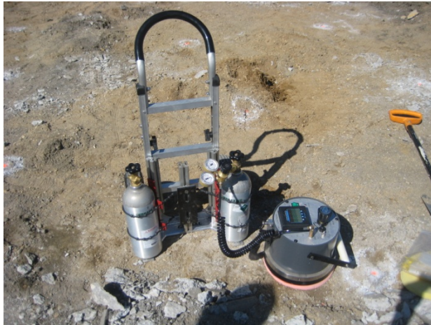
Figure 76. TS2-B: Air permeameter testing device
