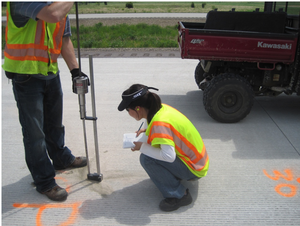
Figure 50. TS3: Collecting DCP data
