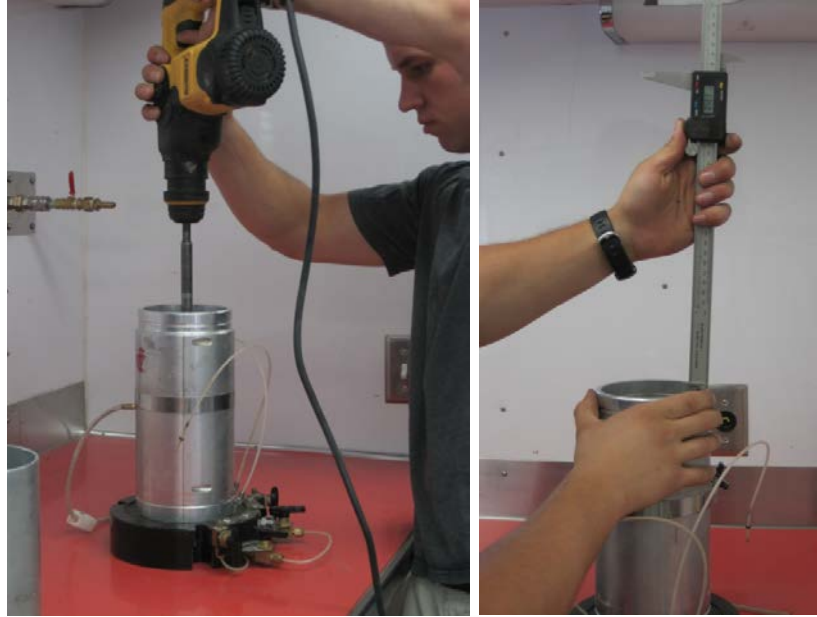
Figure 3. Compaction of a subbase material sample in the split mold (left) and verification of the thickness of each lift using calipers (right)
