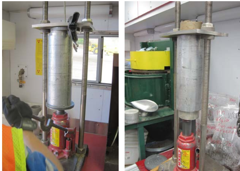
Figure 5. Photos showing the static compaction procedure (left) and sample extrusion procedure (right) of a compacted cohesive soil sample
