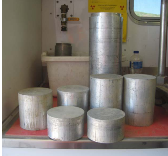
Figure 4. Aluminum spacers (4 in. diameter) used during static compaction
