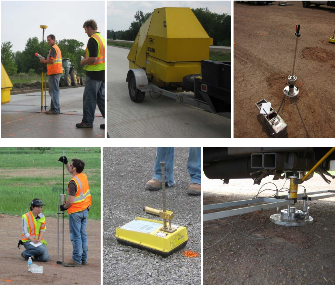
Figure 16. Trimble SPS-881 hand-held GPS receiver, Kuab falling weight deflectometer, and Zorn light weight deflectometer (top row left to right); dynamic cone penetrometer, nuclear gauge; and static plate load test (bottom row left to right)
