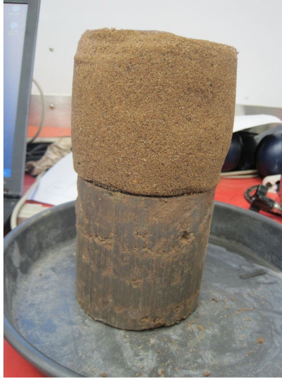
Figure 29. Sand + subgrade layered composite sample extruded sample after shearing
