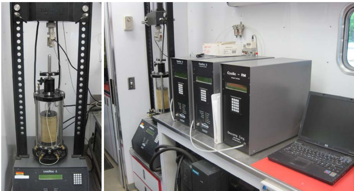
Figure 6. Triaxial chamber, load frame, and computer equipment for resilient modulus tests
