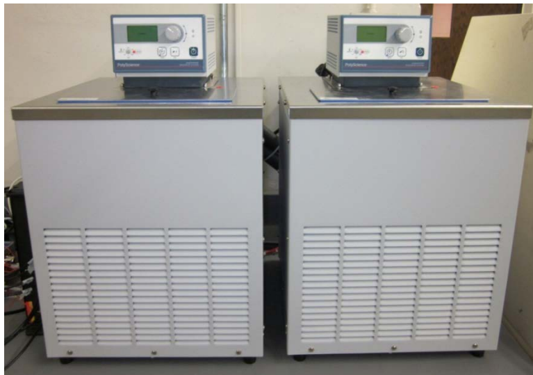
Figure 13. Temperature control water baths used to freeze and thaw samples
