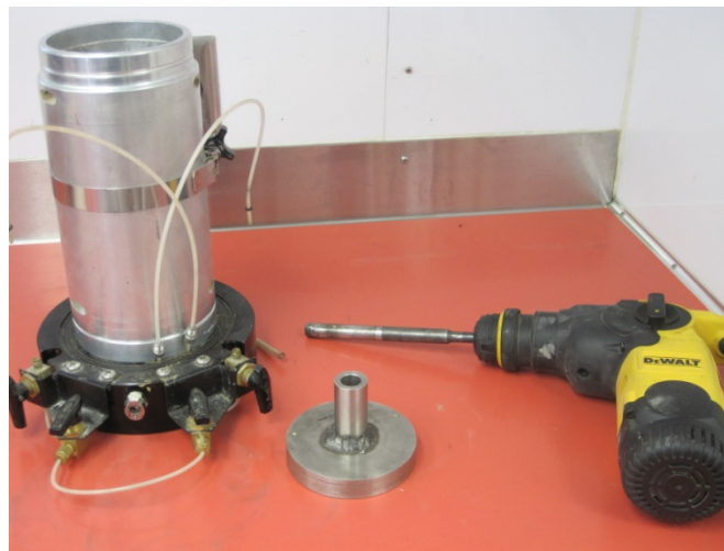
Figure 2. Split mold, steel platen (4 in. diameter), and vibratory hammer for compaction of subbase material samples
