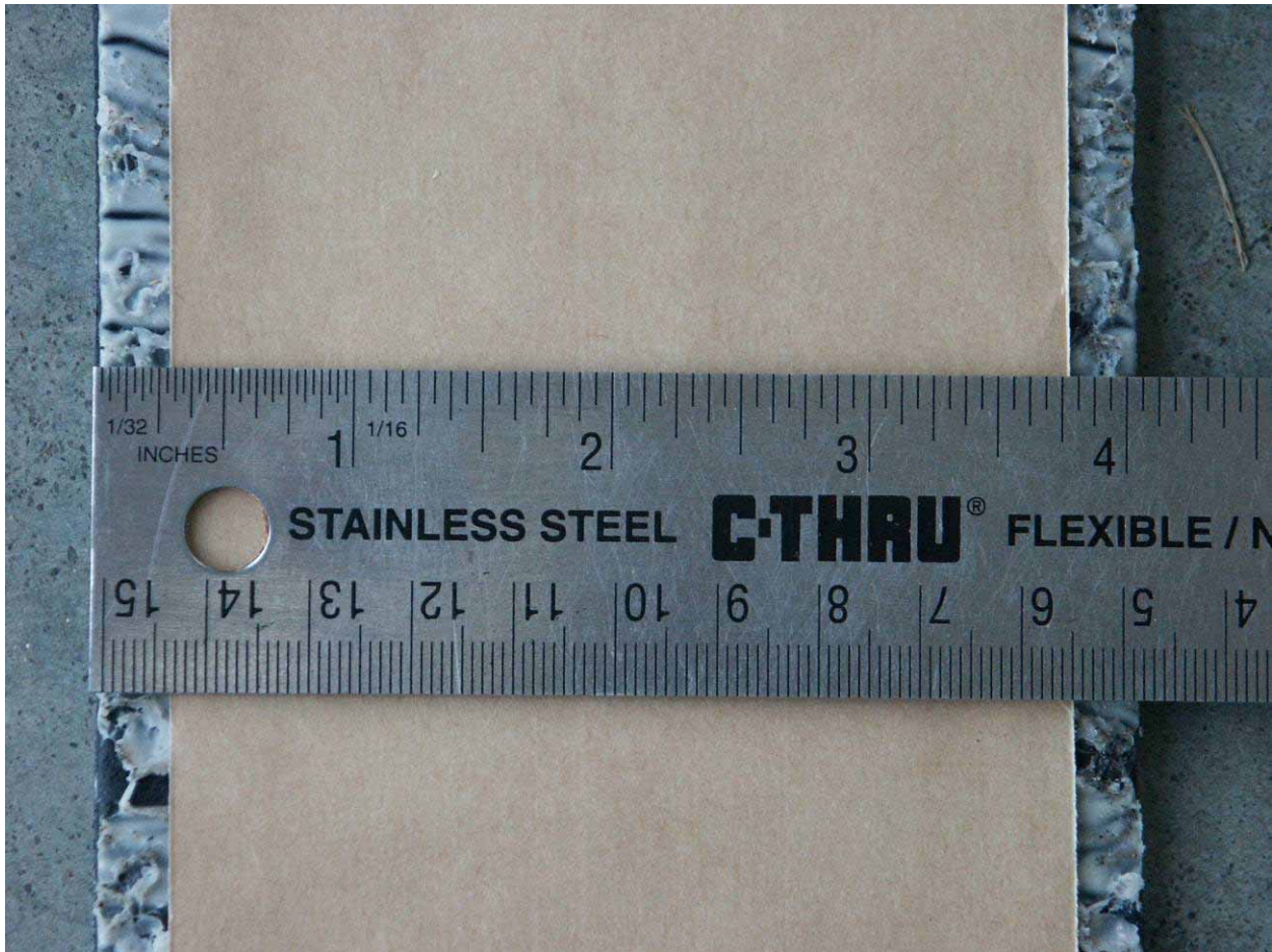
Figure 1. Reverse of the ATM rumble strip with replacement adhesive strip applied.
