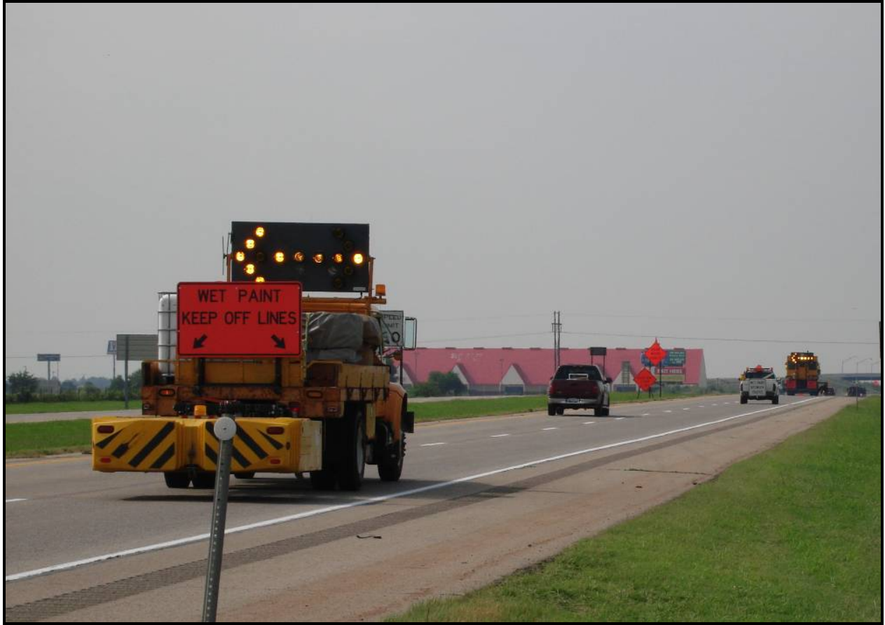
FIGURE 4 Typical advance warning arrows displayed on work convoy shadow vehicles (arrows displayed).
