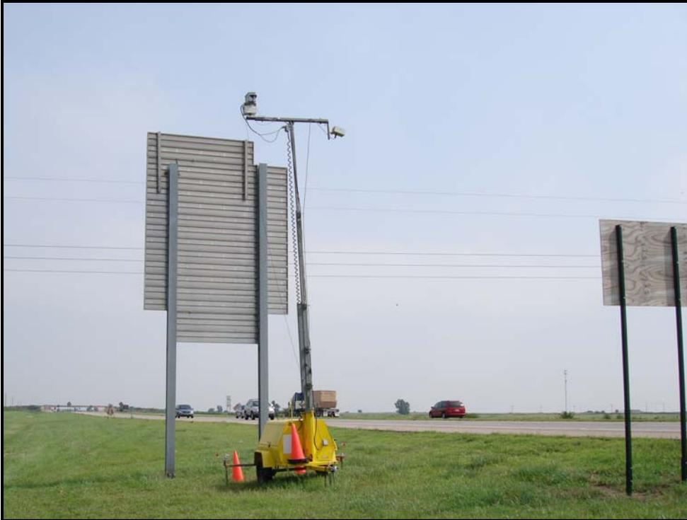
**FIGURE 7** Data collection trailer used for data collection, positioned behind guide sign.
