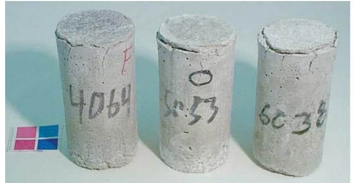
Figure 2. Cylinders exposed to \text{MgCl}_2 solution after 84 days of constant low temperature test. From left to right: 0.40, 0.50, and 0.60 w/c mortar cylinders.
