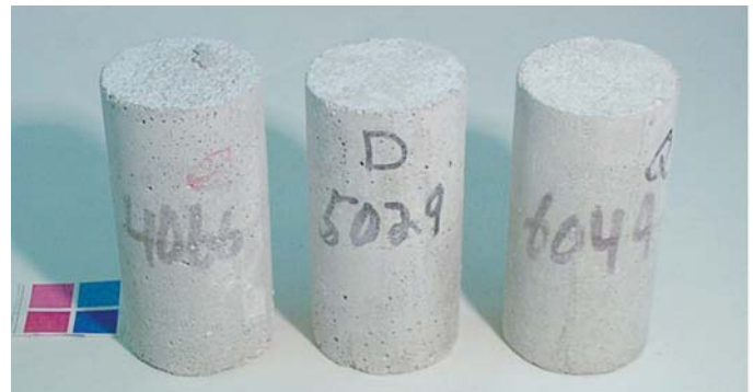
Figure 3. Cylinders exposed to \text{NaCl} solution after 84 days of constant low temperature test. From left to right: 0.40, 0.50, and 0.60 w/c mortar cylinders.
