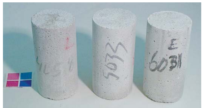
Figure 4. Control cylinders exposed to lime water solution after 84 days of constant low temperature test. From left to right: 0.40, 0.50, and 0.60 w/c mortar cylinders.
