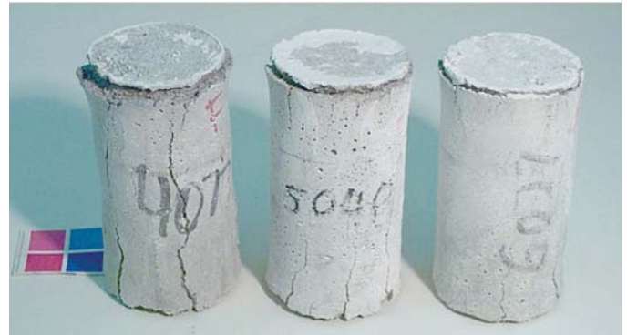
Figure 1. Cylinders exposed to \text{CaCl}_2 solution after 84 days of constant low temperature test. From left to right: 0.40, 0.50, and 0.60 w/c mortar cylinders.
