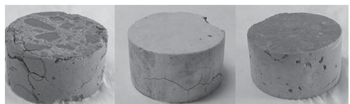
Figure 7. Four-inch [100 mm] diameter 0.45 w/c portland cement concrete specimens after 500 days in high concentration brines. L to r: Samples exposed to CaCl 2 , MgCl 2 , and MBAP brines.
