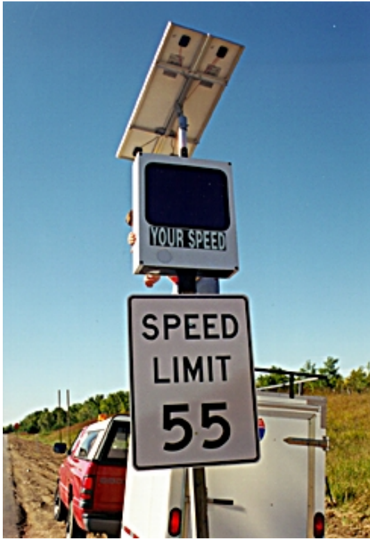
FIGURE 2-6 Speed monitor display mounted on Interstate 35.
