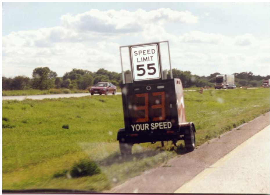
FIGURE 5-2 SpeedGuard radar speed reporting system.
