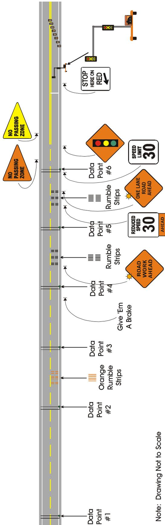
Figure 2. Test Site Traffic Control Diagram
