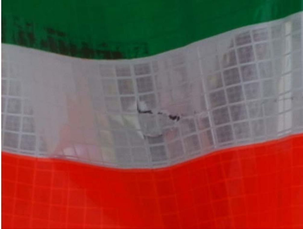
Figure 7. Minor damage to drum sleeve.
