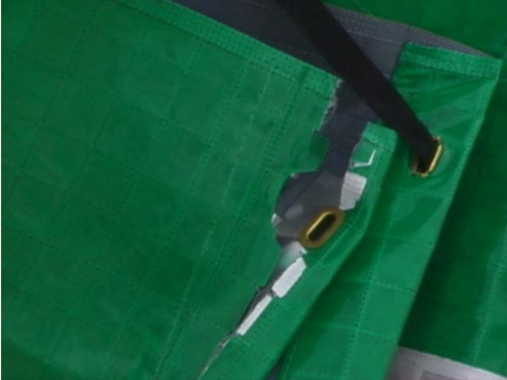
Figure 6. Resulting damage to sleeve on drum that was destroyed.
