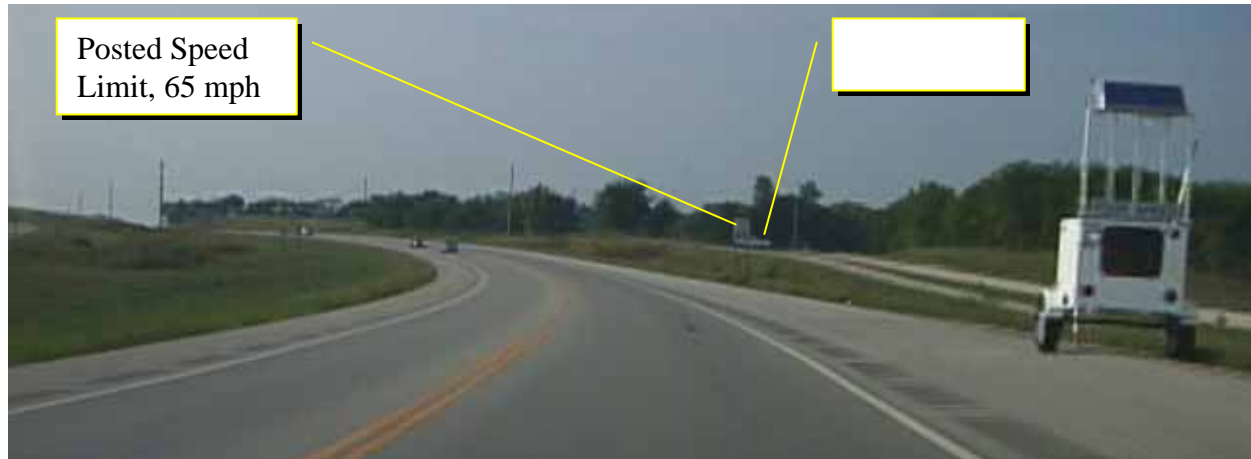
Figure 3. Speed Display, Speed Limit Sign, and Observation Location
