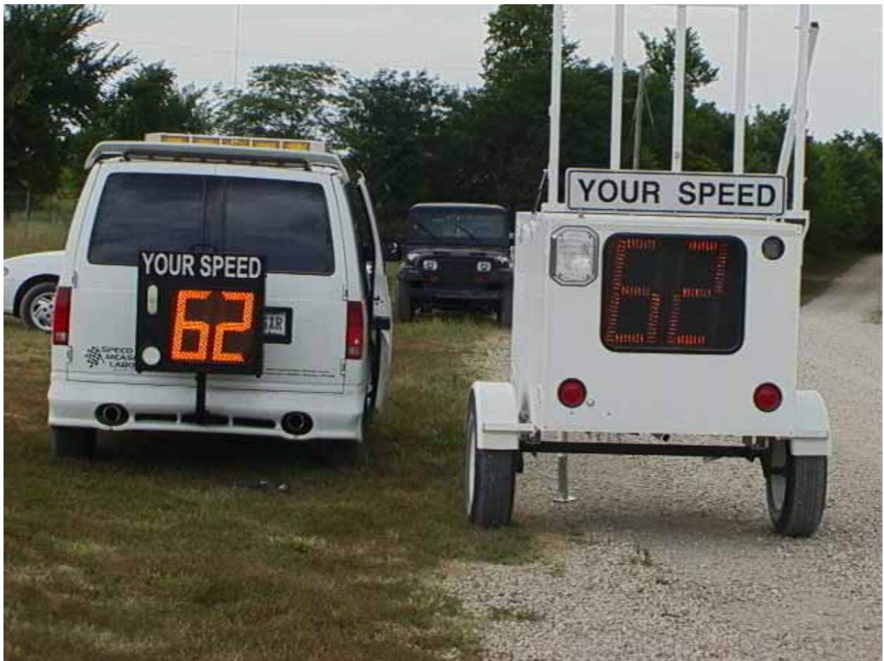
Figure 1. Trailer mount 1 (right) and vehicle/pole mount (left)
