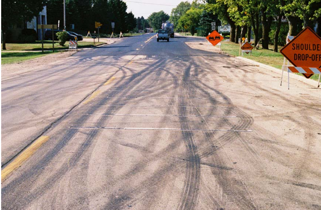
FIGURE 7 WB Test Strip at End of the Day of Psychological Scaling, Viewed Looking Downstream
