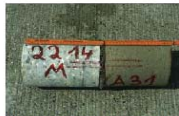
Core showing nonwoven geotextile interlayer between surface concrete (left) and underlying pavement (right) [Cite source]
