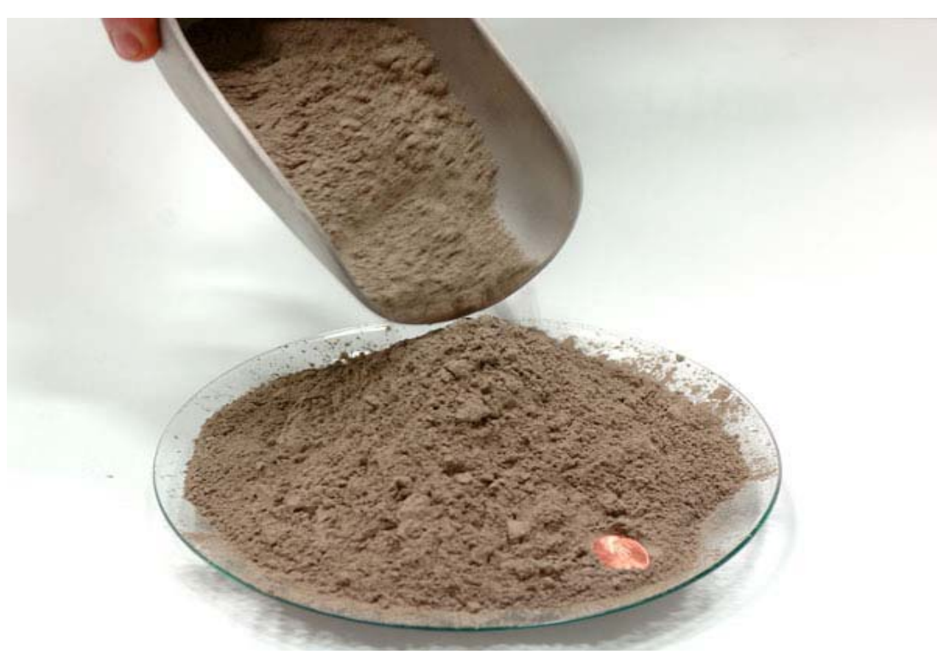
Figure 2. Fly ash, a by-product of coal, is an admixture used in the concrete mix design which possesses pozzolanic properties to increase the strength, workability, and durability of the concrete.
