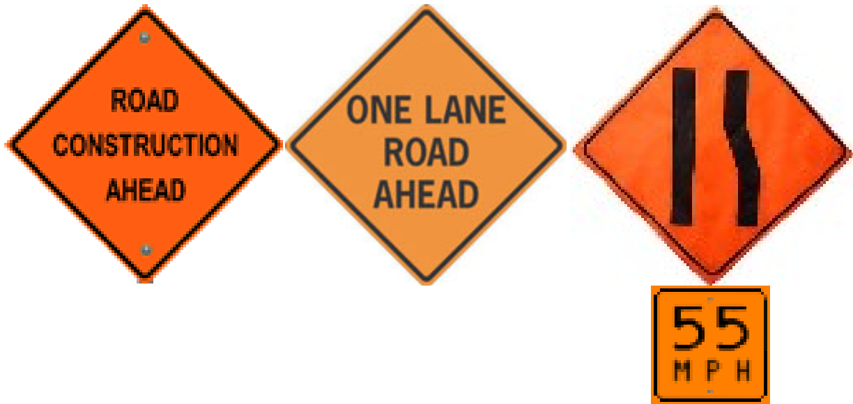
Figure 2. Signs in the advance warning area of the work zone.
