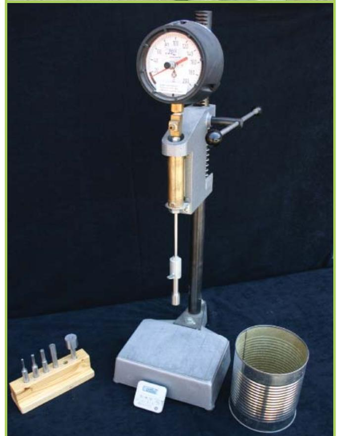
Figure 1. Set time testing equipment
