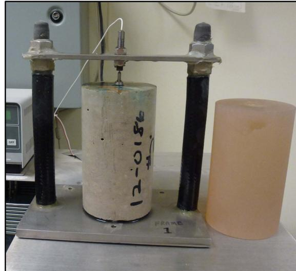
Figure 2: CoTE Test Frame with Sample and Ceramic Cylinder
