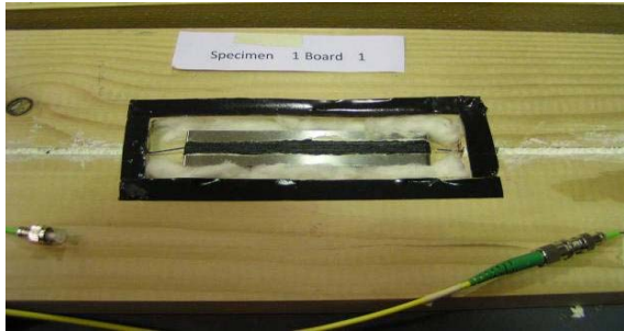
(a) FBG sensor in a recess area and applied adhesive tape.
