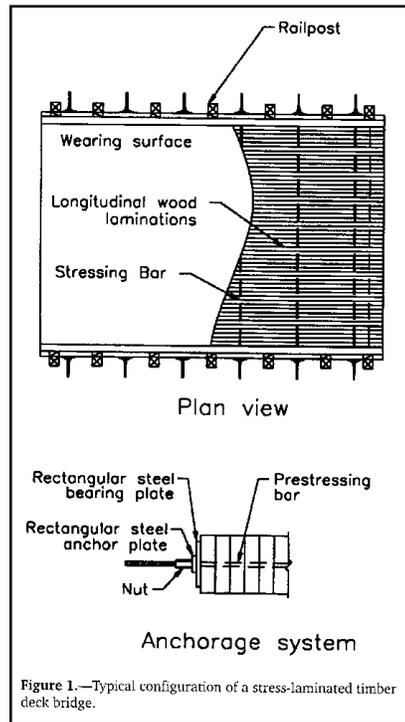
Figure 1.—Typical configuration of a stress-laminated timber deck bridge.
