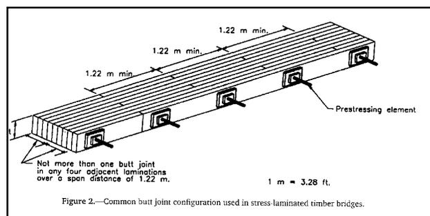
Figure 2.—Common butt joint configuration used in stress-laminated timber bridges.
