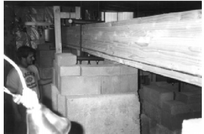
Creep test of FRP-Glulam girders — University of Maine.
