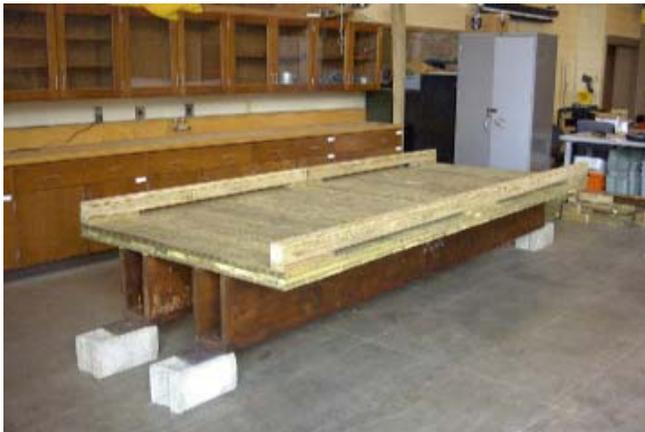
featured 2 LVL box beams supporting a 3-layered deck of 1 1/4-inch southern pine.
