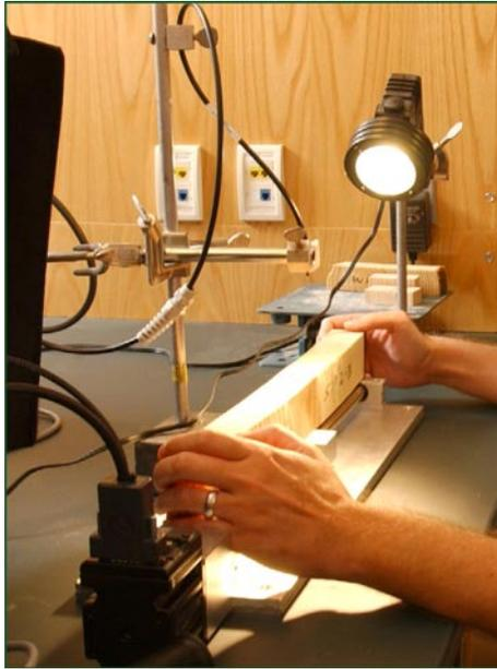
Near-infrared scan of wood specimen.
