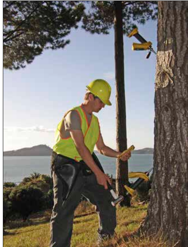
Standing timber being evaluated with a nondestructive testing tool that utilizes ultrasound, lasers, and vibrational characteristics.
