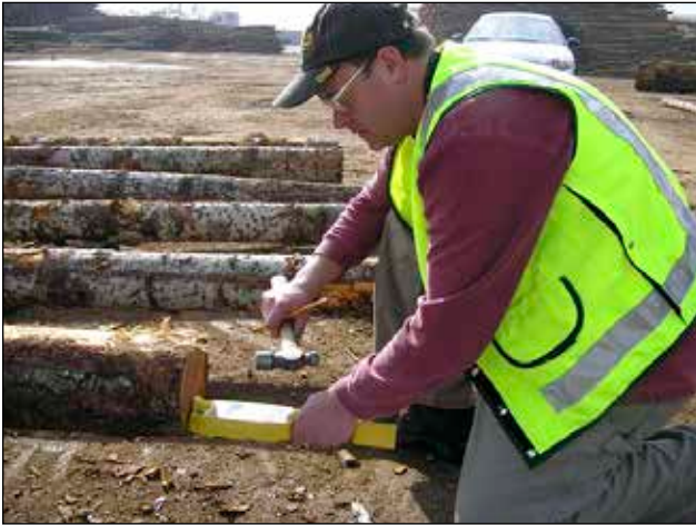
Use of acoustic nondestructive testing tools to evaluate the quality of logs.
