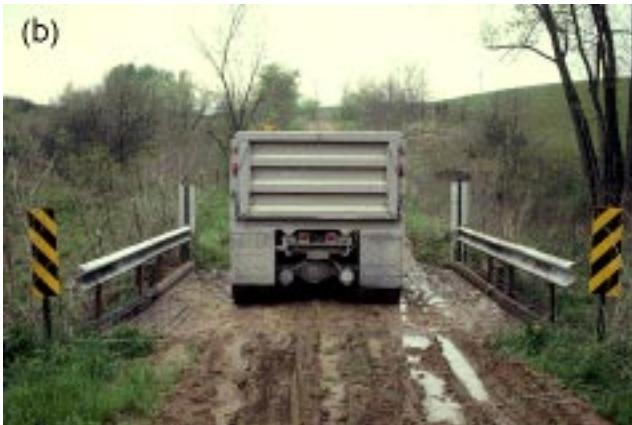
Figure 7—(a) Load position 2 used for the first Dean bridge load test (looking north). (b) Load position 1 used for the second Hibbsville load test (looking west).
