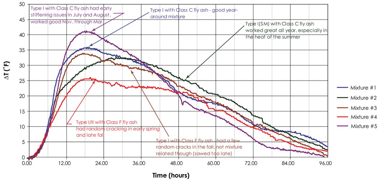
Figure 2. Qualitative comparison of heat signature curves during the mixture design stage
