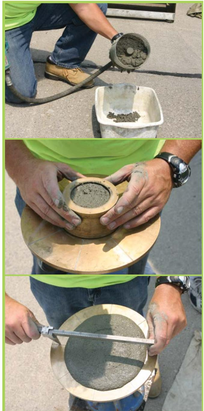
Figure 1. Mortar flow testing equipment
